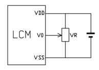
V<sub>DD~</sub>V<sub>0</sub>: LCD Driving voltage VR: 10k~20k
